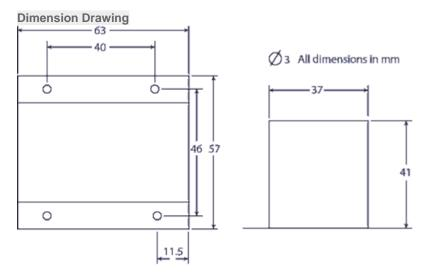
Dimensions are for case only. Connectors and controls are not included
