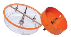
High speed holesaws for cutting precise neat holes into plasterboard, plywood & acrylic sheet (not recommended for cutting metal). Suitable for power drills with a standard 3/8" chuck. T 2312A Cuts hole for One-Shot® 100mm speaker & grill combinations. For 200mm speakers, use the T 2314A adjustable model.
