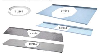
Designed to be installed with the "One-Shot"® ceiling speakers, these pans support the ceiling tile to minimise sag and reduce damage to soft tiles. Fits inside the "T-bars" for maximum support for the tile. Recommended for use with mineral fibre and acoustic ceiling tiles.
